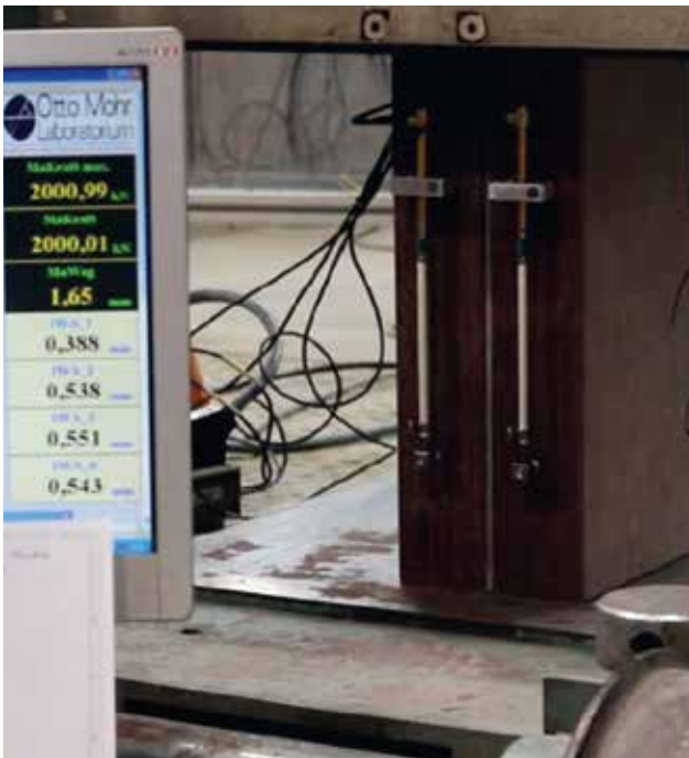
Fig. 8) Compression test at Otto-Mohr-Laboratory, TUD
